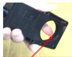
Clean debris from slot in bottom of valve body. Valve slide must be able to slide to bottom.
